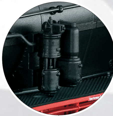
Knorr design simple feed pump on the left running board
