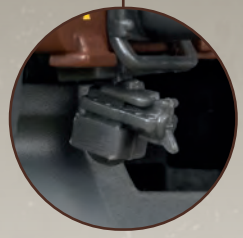
The heating socket is separately applied below the buffer beam.
