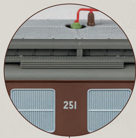
Additional air intake box on the right-hand side of the loco.
